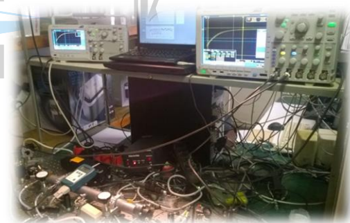
Fig. 3. The developed CRDS system capable of time resolved measurement of acetone concentration with 1 ppm resolution.
